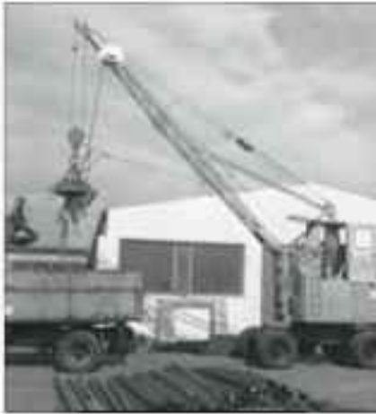
1962: rope-driven 5833 with elevated operator cab
